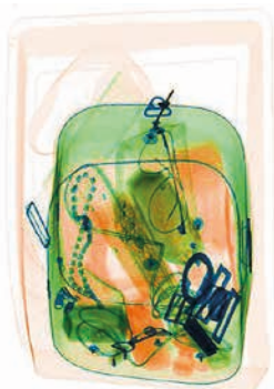
Excellent image quality. Organic materials shown in orange, metal in blue and a mix of them in green.
